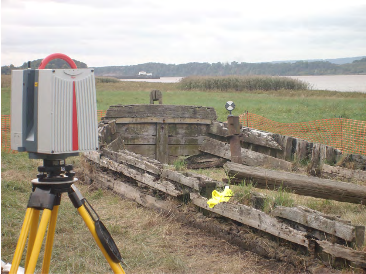
Fig. 1 Laser scanning of the Harriett with the Leica HDS6000
