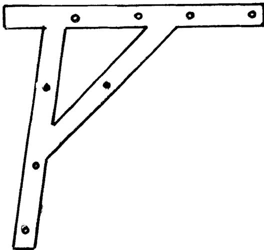
Figure 4. Braced knee, Seppings' version with 'tail'.
