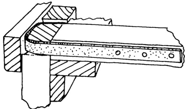
Figure 10. Staple knee found on wreck site SL10 on the Slufter survey.
