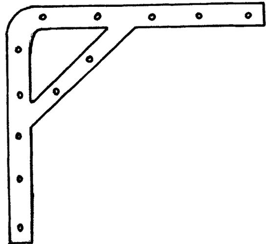
Figure 5. Braced knee, Seppings' second variant with curved end.
